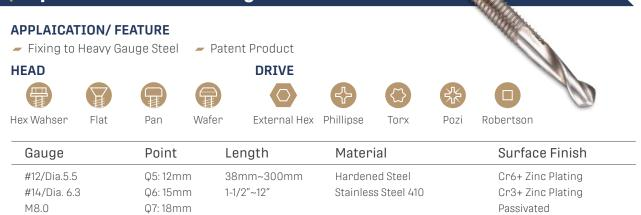
Bi-Metal Spiral Point Self-Drilling Screws
